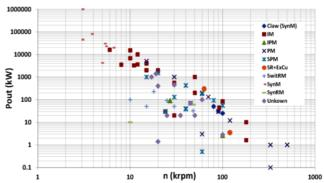
Fig. 2. Survey of high-speed machines by topology [1].
