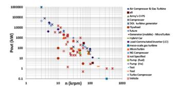
Fig. 1. Survey of high-speed machines by application[1].
